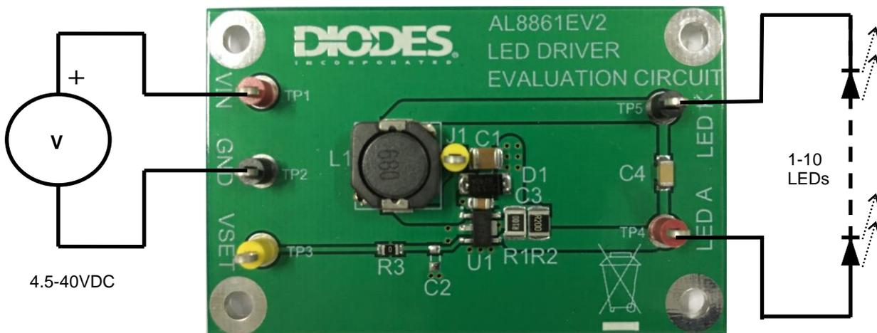
Figure 1: AL8861EV2 evaluation board and connection diagram
