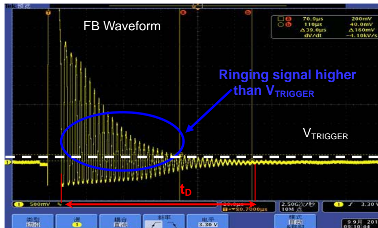
Figure 4. The Ring Signal of FB Pin
